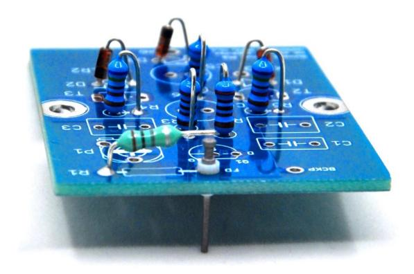
Continue by installing the FET transistor. I chose the original BC264, whose GATE leg is on its edge. If you choose another FET, keep in mind that the GATE leg may be elsewhere. Always check this against the data sheet of the particular FET transistor. Note that the GATE leg is also soldered in the air to the teflon pin.
