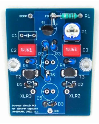
Two electrolytic capacitors remain to be installed.
