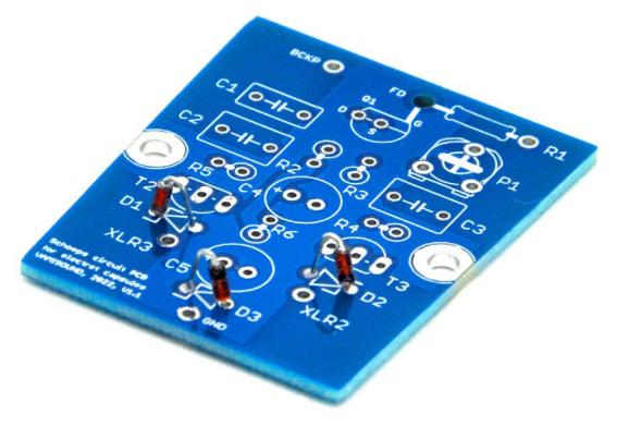
Continue by soldering resistors as in the picture. R2 and R3 form a matched pair, the same for R4 and R5.
