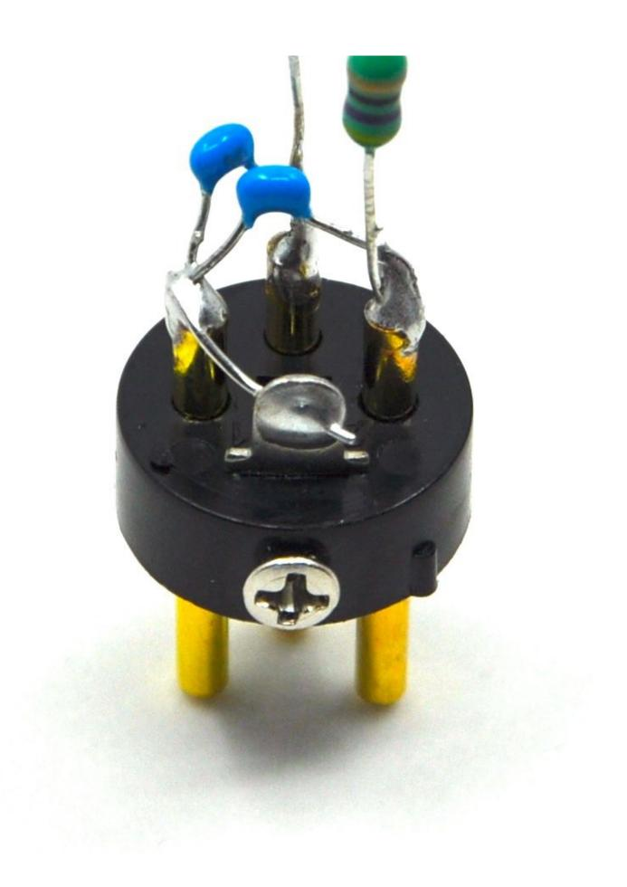
What must be added is that the microphone can function even without this filter. So there is nothing stopping you from trying the microphone without it. In this case, just connect pin 1 of the XLR connector to the GND pad on the board, pin 2 to the XLR 2 pad on the board and pin 3 to the XLR 3 pad on the board using a cable. If you have a problem with signal interference, you can finish the filter later.
