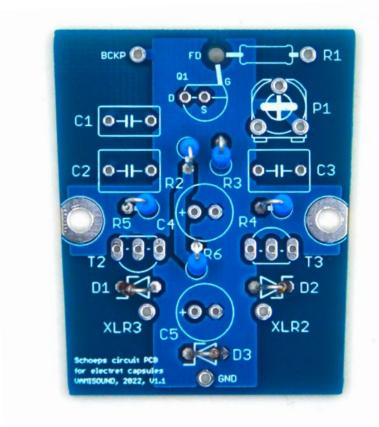
Install the teflon pin and the remaining R1 that feeds into it as if in air.
