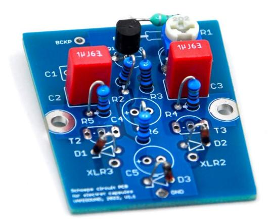
Continue with the installation of two transistors T2 and T3. Before that, match the HFE parameter on these transistors. Most multimeters have a socket for the transistors and can therefore measure the base HFE parameter.
