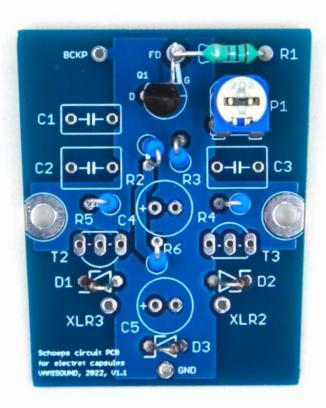
Now solder the two film capacitors. Note that the C1 position remains unoccupied. C1 forms the LPF for very bright capsules. You can experiment with values of round 22nF if needed.
