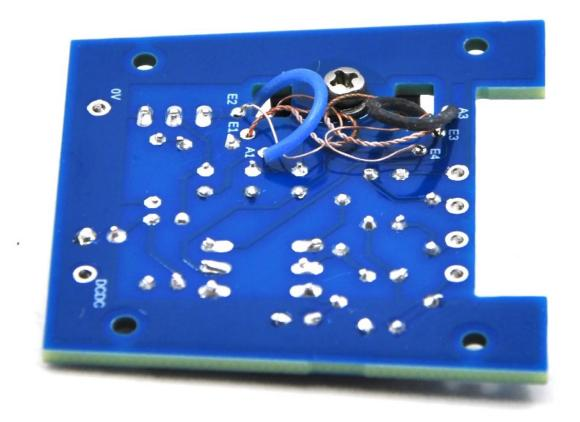
Install all three switches in their positions. Solder them slowly. Take your time. They don't like a lot of heat. On the large polar pattern switch, remove the one ground leg that runs from the switch chassis to better position the switch on the board.
