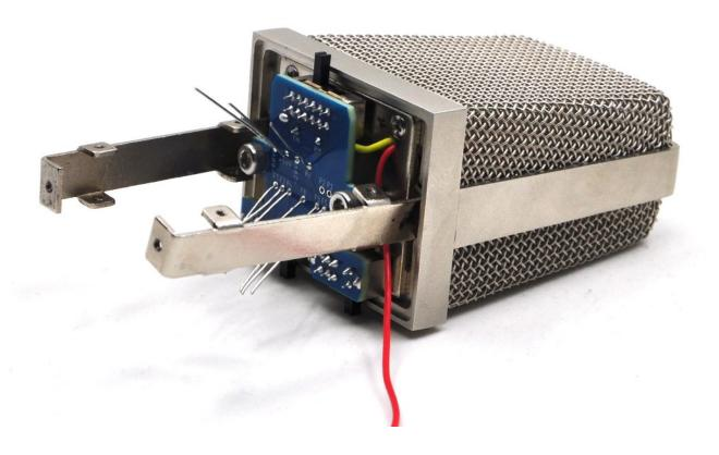
Solder two 40 mm long wires to the OV and DCDC pads on the transformer board, which will be used later to connect to the DC-DC converter board.
