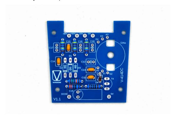
All that's left is to install the diodes, transistor and one electrolytic capacitor. Again, watch out for its plus and minus legs.
