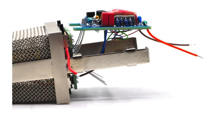
Secure the plate with 4 pcs of 6 mm long M1.8 screws.
