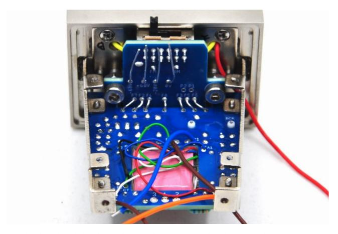
From the other side of the board, carefully cut off the excess resistor legs that were used for interconnection.
