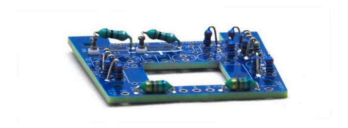
The preprinted component outlines on the circuit board will help you. Bend the legs in a similar way as indicated.
