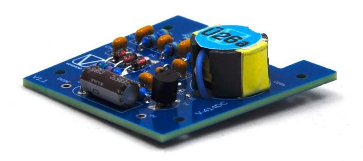
Screw the transformer to the back of the board with a 6 mm long M2 screw. If you have screw glue, use it and fix the screw. This will prevent it from coming loose later.
