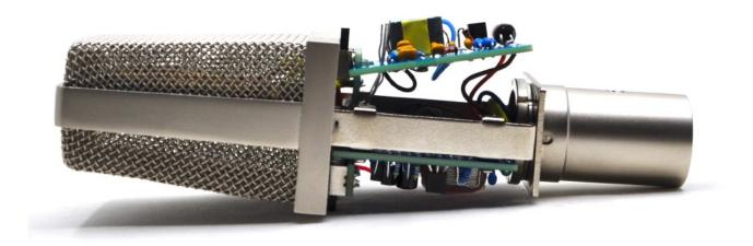
Pull the DC-DC converter board carefully against the chassis. Pull the resistor legs together to prevent a short circuit inside. Make sure there is no pinched cable anywhere before screwing the board firmly to the chassis using 4 M1.8 screws with a length of 6 mm.
