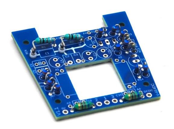
Install the 2SK3OA-O input FET transistor with its middle leg leading to the teflon pin nearby. Everything is as if in the air, nothing touches the pcb surface.
