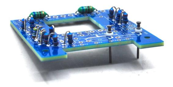
Cut off the excess parts of teflon pin with pliers as shown in the picture.
