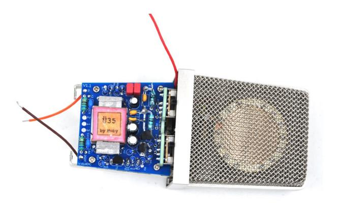
Now carefully solder the 7 resistor legs from the inside to connect the switch board with the transformer board. Visually check that these connections are OK, there is no contact between the legs or to the chassis.
