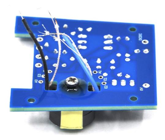
Now CAREFULLY solder the wires to the board. Note where the blue wire is and where the black wire is.
