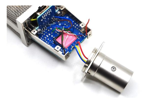
Carefully screw the XLR part of the microphone body to the rest of the chassis.
