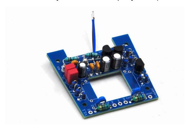
At this stage it is possible to give the whole board a final cleaning with isopropyl alcohol to make everything perfectly clean. Don't underestimate cleaning!
