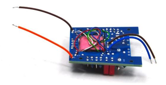
Now take the prepared transformer board and place it on the 7 resistor legs that stick out of the switch board. Carefully slide it in.
