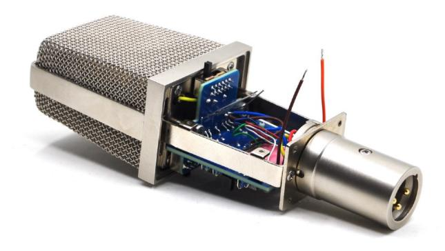
Now carefully slide the DC-DC converter board onto the 5 resistor legs that lead on the other side from the switch board. Also solder the two cables leading from the transformer board to the DCDC and OV pads on the DC-DC converter board.
