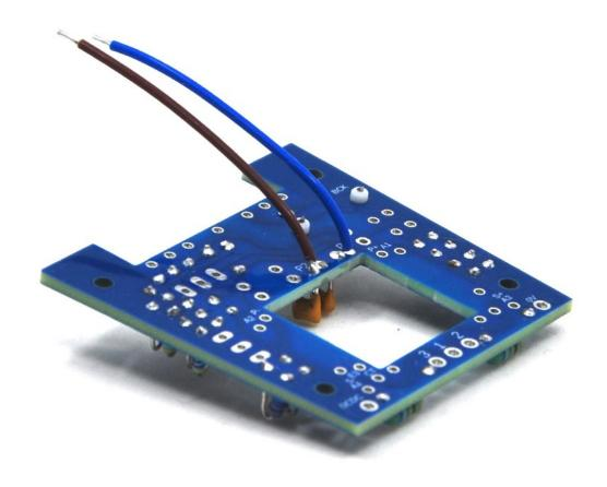
Solder the remaining transistors and the two blue capacitors C9 and C10.
