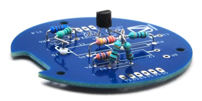
Now solder the BC557B transistor. Be cautious of its correct orientation.
