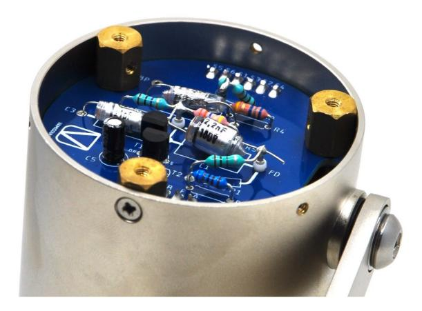
Carefully connect the two wires from the capsule to the HiZ board. The cable from the front diaphragm goes to the "FD" teflon pin on the HiZ board. Backplate wire from the capsule to the "BCKP" pad on the HiZ board.
