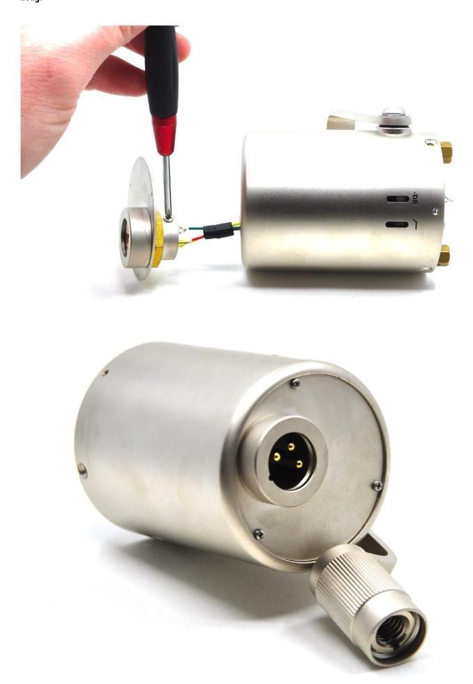
Screw the whole set of plates to the microphone body tube with three screws.
