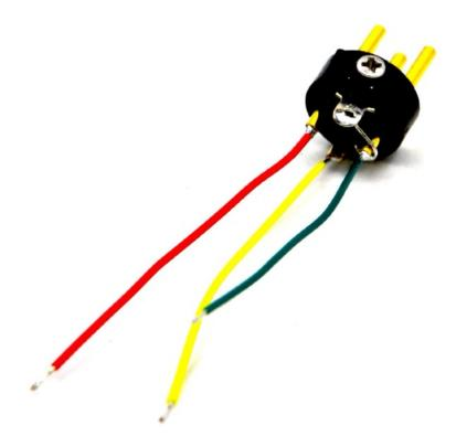
Connect the so prepared connector insert to the transformer pcb, to the pads marked 1, 2 and 3. XLR1 to pad 1, XLR2 to pad 2 and XLR3 to pad 3. Also note that three M2.5 spacers of 17mm length have been installed on the main parts pcb. These two interconnected boards are now holding together nicely.
