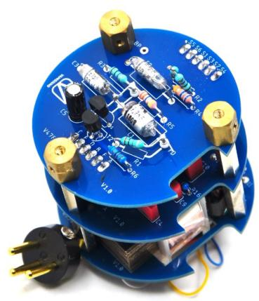
Insert the assembled plates into the microphone body. Before doing so, unscrew the bottom metal plate from the body.
