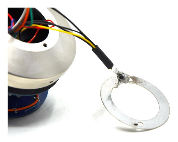
Attach the grounding ring to the body and temporarily screw it on using one screw. Route all cables through this earth ring to the outside. That screw with the eyelet and cables is now hidden inside the body.
