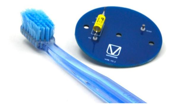
From the bottom strap, solder 3 cables about 5cm long to the teflon pins. Shunt the remaining part of the teflon pins. Clean these connections again.
