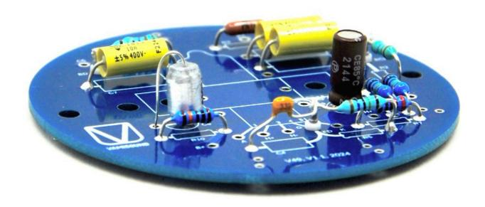
Now it's time to carefully wash the pcb with a brush and isopropyl alcohol. Make sure everything is clean and free of flux from soldering. Especially focus on the teflon pins and the connections to them. Be careful especially around the polystyrene capacitor which don't like the isopropyl alcohol.
