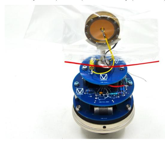
Screw the capsule pcb to two spacer posts. The cables that stick out from the bottom have to be connected now to the main parts pcb.
