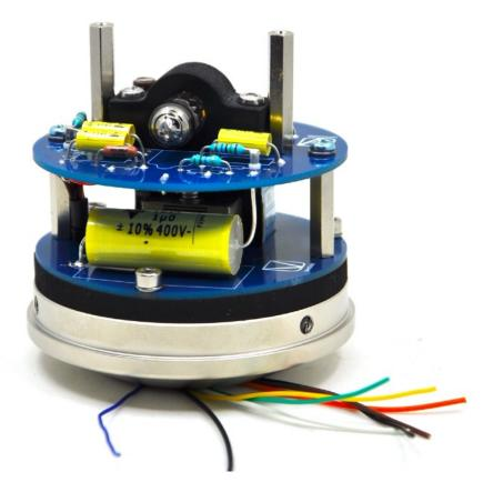
Make sure that all cables are routed through the hole in the bottom of the M49 body and are not pinched anywhere.
