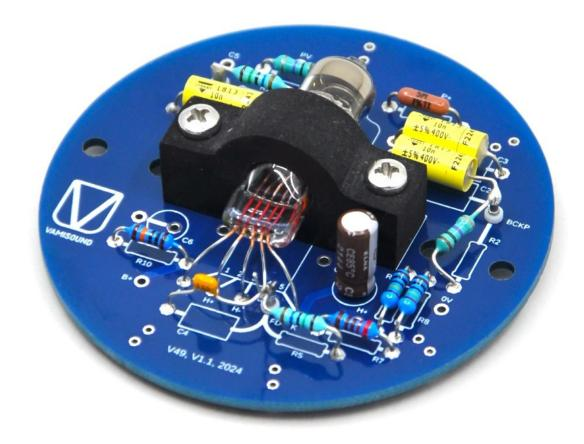
The tube grid is connected in air to a teflon pin to which resistor R5 and capacitor C4 are already connected.
