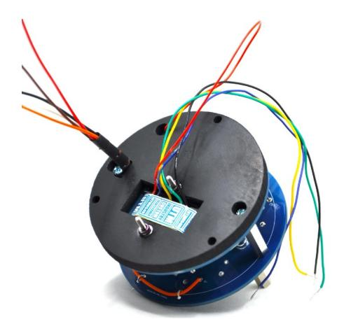
Now connect the red cable that runs from the "P+" pad on the main parts pcb to the "P+" pad on the transformer pcb near the C5 leg of the capacitor.
