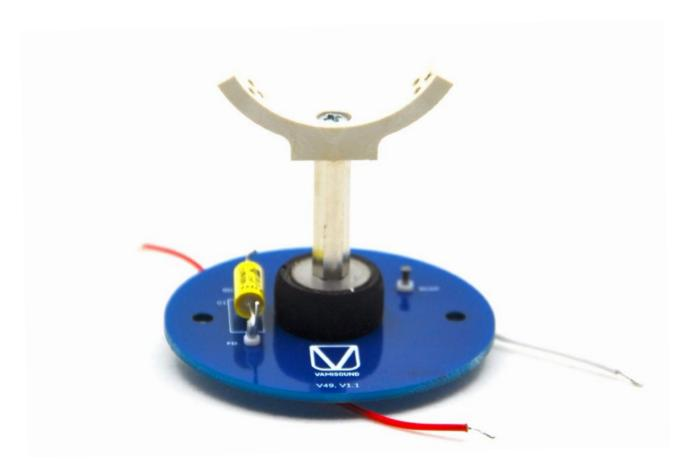
Carefully install the caspsule in place and immediately cover it with the protective bag.
