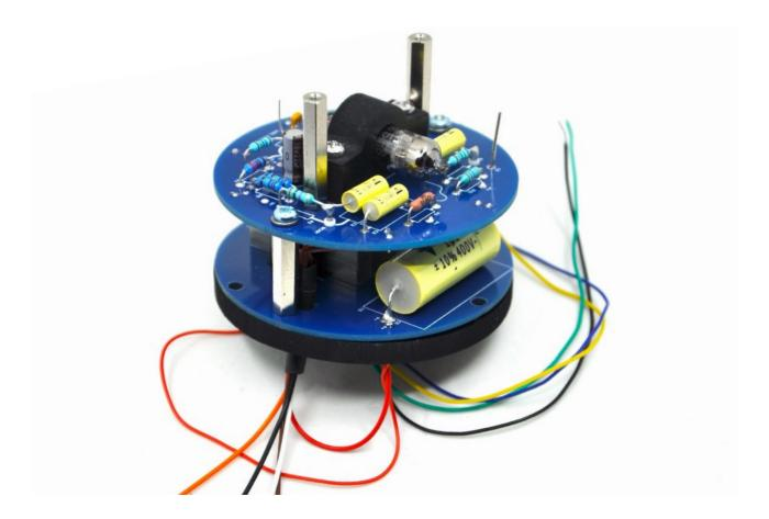
Screw both pcb to the bottom circular part of the M49 style body. Use 3 pieces of M3 screws about 10mm long. Use washers. Solder second C5 leg into the main parts pcb.
