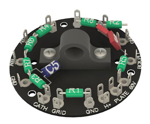
Insert the tube into the rubber holder as you see in the picture. Check with the datasheet of the particular tube you are using to see which wire leads are which. Accordingly, connect the leads from the tube to the appropriate lugs/eyelets on the main parts board. Heater to H+ lug/eyelet, heater ground to GND lug/eyelet, ANODE of the tube to PLATE lug/eyelet, CATHODE of the tube to CATH lug/eyelet on the main parts board.
